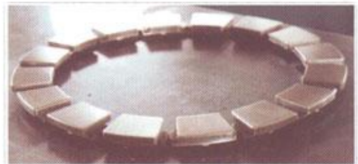
ONE SET OF SMALLEST PADS OF STEAM TURBINE
