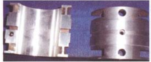
MOTOR BEARING - 200mm BORE
