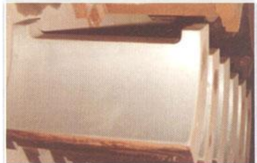
JOURNAL PADS OF STEAM TURBINE
