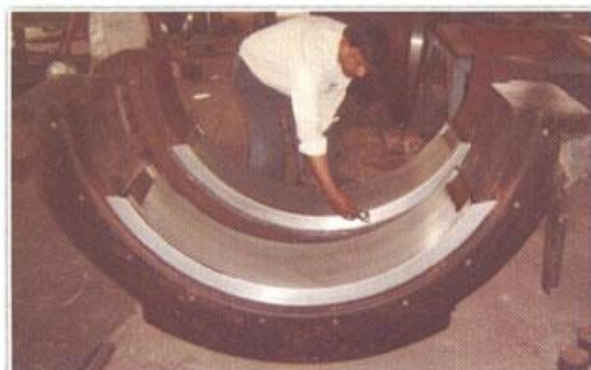
COAL MILL LINER FOR POWER PLANT
